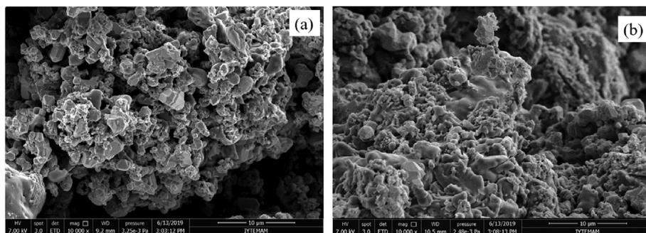
**Fig. 5** – Surface morphologies of LSCF coating layers as deposited on GDC electrolyte. (a) Sample 4, and (b) Sample 5. Nozzle to substrate distance was 23 mm and 11 kV voltage was applied while the ceramic electrolyte specimen was heated at 400 °C.
