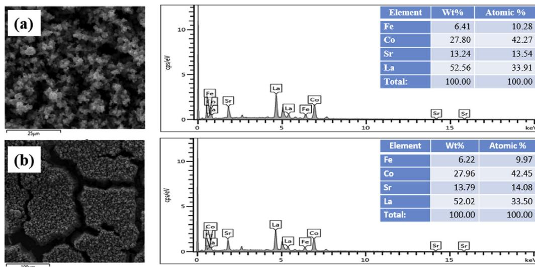
**Fig. 7** – EDX analysis performed on samples with (a) coral (micro porous) surface coded “4” and (b) cracked (macro porous) surface of sample coded “7”. Elemental composition of electro-sprayed samples in atomic % and weight % were determined by semi-quantitative EDS analysis.
