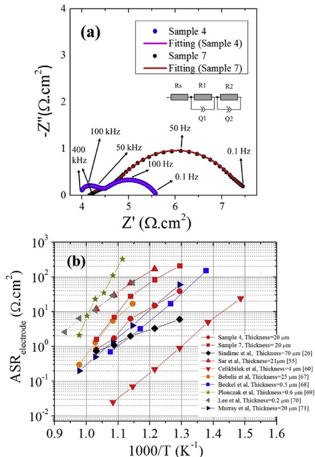
**Fig. 9 – (a) Nyquist plots of EIS data for Sample 4 and 7 obtained at 700 °C. The equivalent circuit model used for fit is shown as inset. Obtained impedance data and summit frequencies are also included (b) Temperature dependence of  $ASR_{pol}$  ( $ASR_{electrode}$ ) for the deposited films from Samples 4 and 7. The electrode polarization resistance data obtained by other methods are also included for comparison.**
