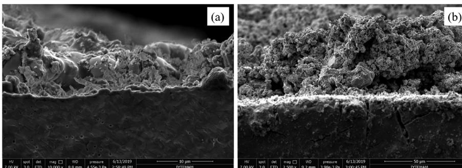
**Fig. 4 – Cross sectional views of coated electrolyte. Top half of image shows the LSCF coating and GDC substrate. Surface morphologies of LSCF layers as deposited on GDC electrolyte. (a) Sample 3 and (b) sample 4.**
