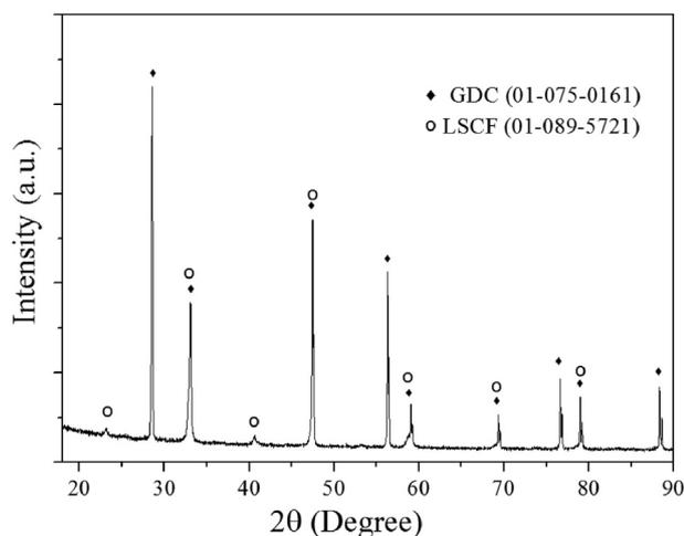
**Fig. 8** – X-ray diffraction pattern of LSCF coated GDC symmetrical cell specimen (Sample 4). CuK $\alpha$  radiation was used in analysis. Peaks corresponding to LSCF and GDC phases are marked by ○ and ◆, respectively.
