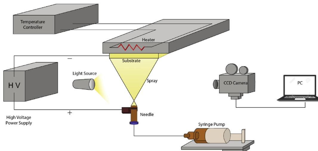
**Fig. 1 – Sketch of the ESD set-up. Electrolyte specimen (substrate) sits upside down on the heated metal plate on which there is a 10 mm diameter hole. Potential difference between the heated metal plate and the needle draws the solution onto the target ceramic specimen.**
